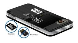
**Note:** The Samsung A867 has been tested to support up to an 8GB memory card.
