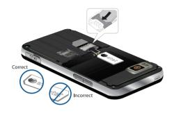
Note: If the card is not inserted correctly, the phone does not detect the SIM card. Re-orient the card back into the slot.
