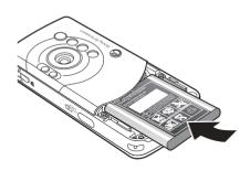
3 Insert the battery with the label side up and the connectors facing each other.
