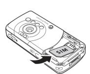
2 Slide the SmartChip into its holder with the gold contacts facing down.
