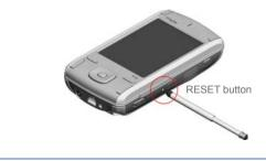
**Warning!** Always turn off your device before performing a soft reset or installing/replacing the battery and SIM card.
